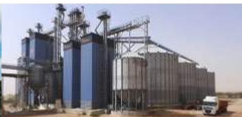
STORAGE : PADDY RICE Senegal Silos X8 Rotary cleaners X2 Dryers bin X4 Handling equipment
