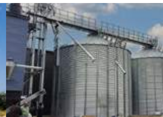
DRYING STORAGE Silos X2 Drying bin Fixed loading Unloading Biomass heater
